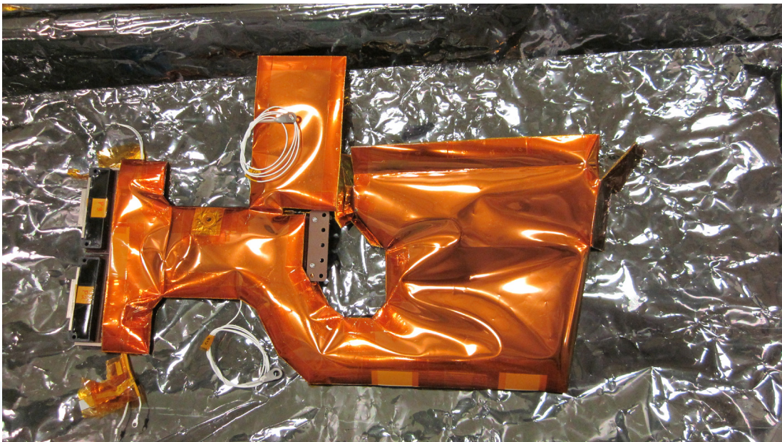
MLI Blanket Installed
