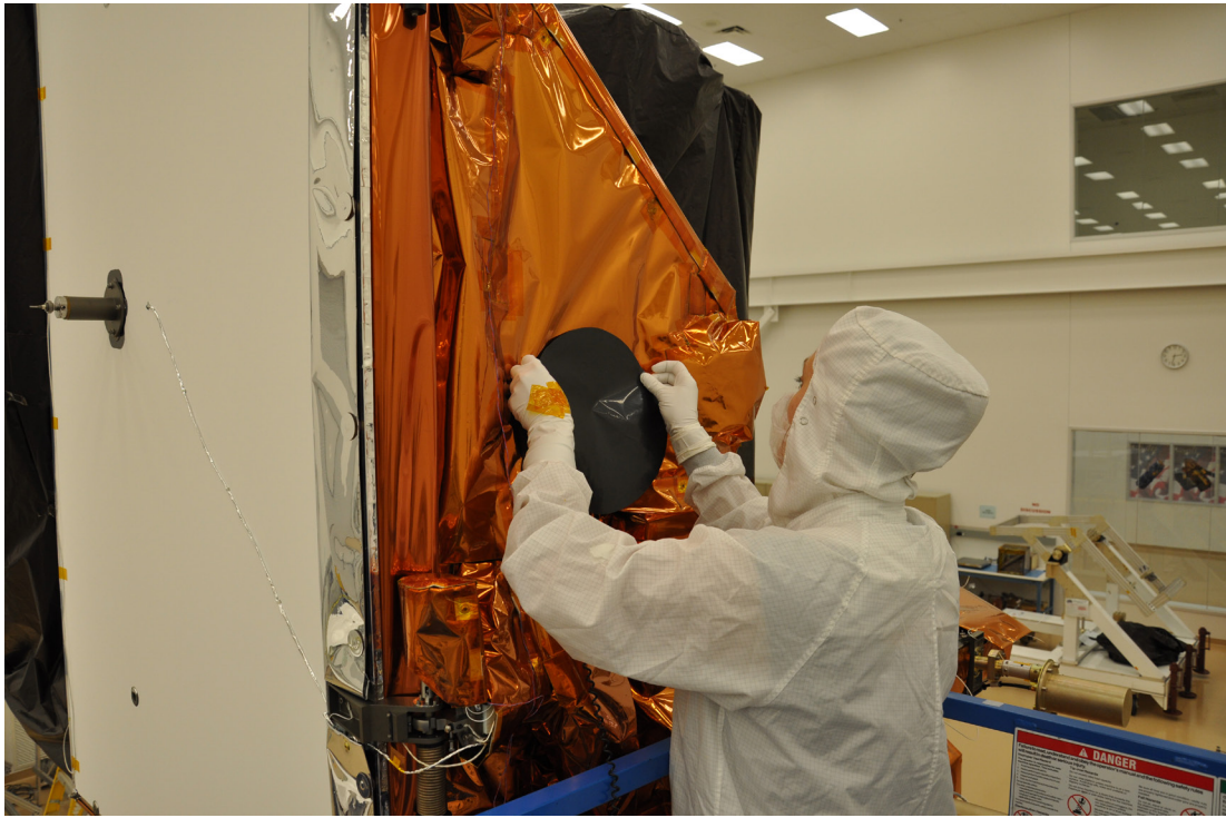
MLI Blanket Installation
